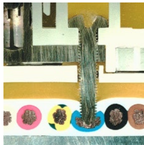
Fig. 2: Microsection of a contact point
